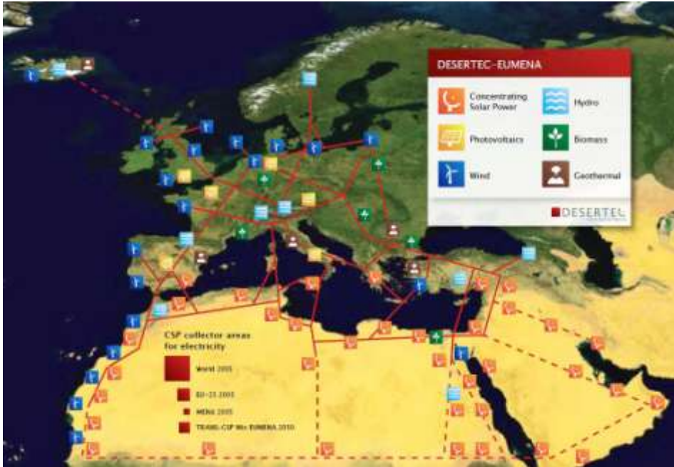
Figure 5. DESERTEC: An Intercontinental super grid system connects Geothermal power in Iceland with solar energy in North Africa and Saudi Arabia. Storage and power is listed as hydro-electricity and molten salt thermal stores for solar installations. Biomass, Hydro, Gas, and storage are all modest compared to wind and solar and serve as their Hybrid partners.
