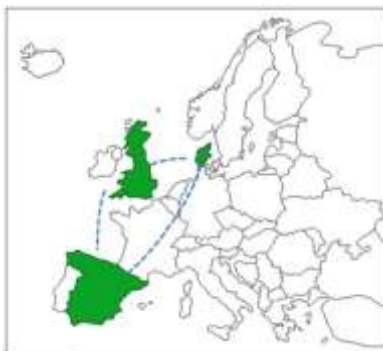
Figure 4. High Voltage DC transmission lines, by land and sea could link the UK, Denmark, and Spain to swap or store renewable energy. Systems with a 20GW peak would need transmission capacity of 4GW on each line.
