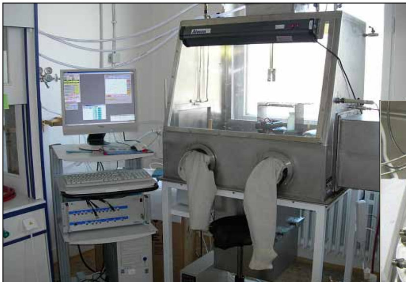
Two nitrogen glove-boxes with built-in electrolysers sealed by removable flange.
