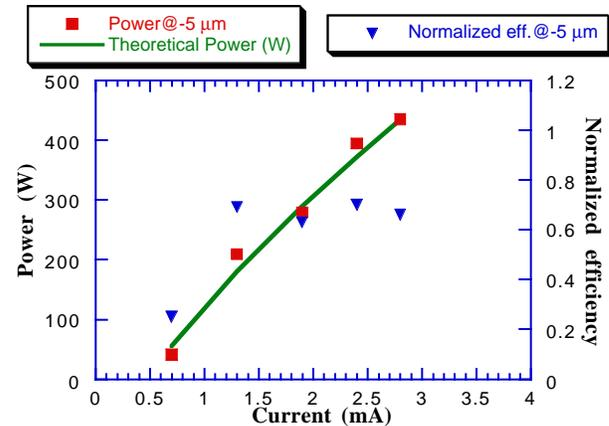
Figure 3. Power at a cavity detuning of  $-5 \mu\text{m}$  from the synchronous length and the efficiency divided by  $4N$ . The theoretical model assumes constant bunch length and emittance and energy spread proportional to the square root of the charge per bunch.
