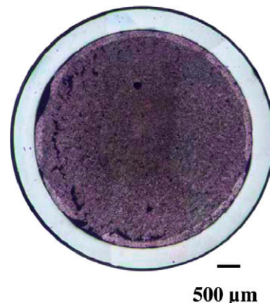
Fig. 4. Cross-sectional photomicrograph AFC-1F Composition A1F4 (U–29Pu–4Am–2Np–30Zr) irradiated to 6.8 \times 10^{20} fissions/cm 3 (approximately 6.0 at.%).
